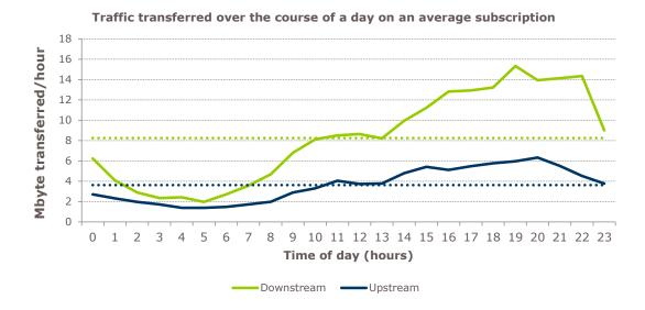
Figure 9. Average volume of traffic transferred on an access connection per hour (measured on the ISP B network in November 2013).
