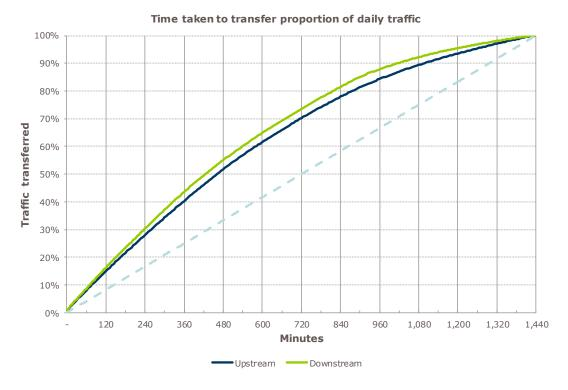
Figure 10. The cumulative proportion of total traffic volume transferred in a day by minutes (measured on the ISP B network in November 2013)
